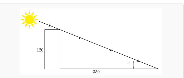
We see that the triangle formed from the height of the building, the ground, and the ray of sunlight creates a right-angled triangle. The angle we want, x, has an opposite side length of 120ft and an adjacent side length of 350ft. Since we have sides O and A, we use the TOA in SOH CAH TOA, which tells us
