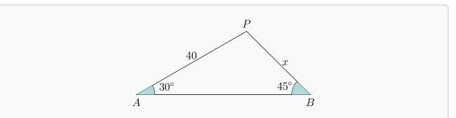
We recognise that the missing side length x is part of the side-angle pair with 30°, while the 40 and 45° form a complete side-angle pair. Noticing these side-angle pairs should tell us that it is probably helpful to use the Sine Law, which says
